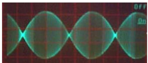
The picture shows the waveform of a well adjusted PSK31 signal, which resembles the waveform of a two-tone test, used for measuring PEP power in SSB.
